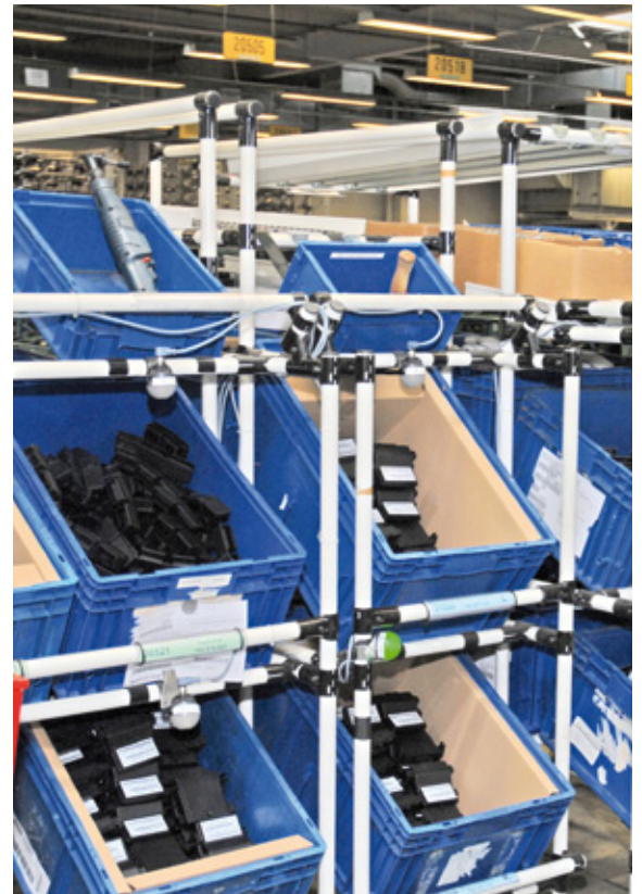
The light signal marks the box with the component that is next to install
