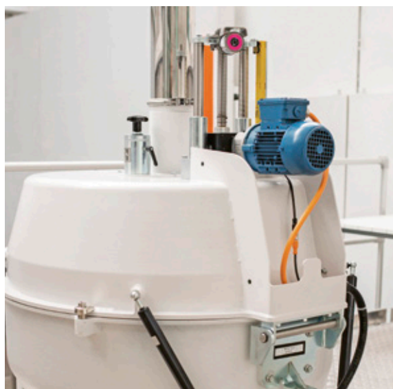
The MHS huller in the Milling Solutions Technology Center at Bühler AG: An impact ring moves up and down under the cover during the hulling process
