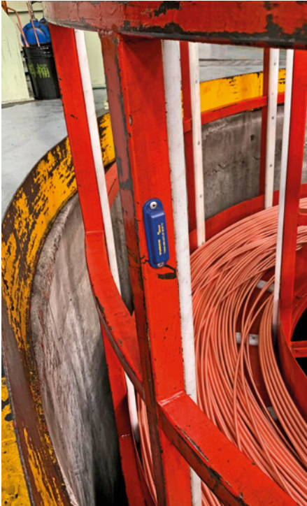
The robust UHF tag can be mounted directly on the metal frame
