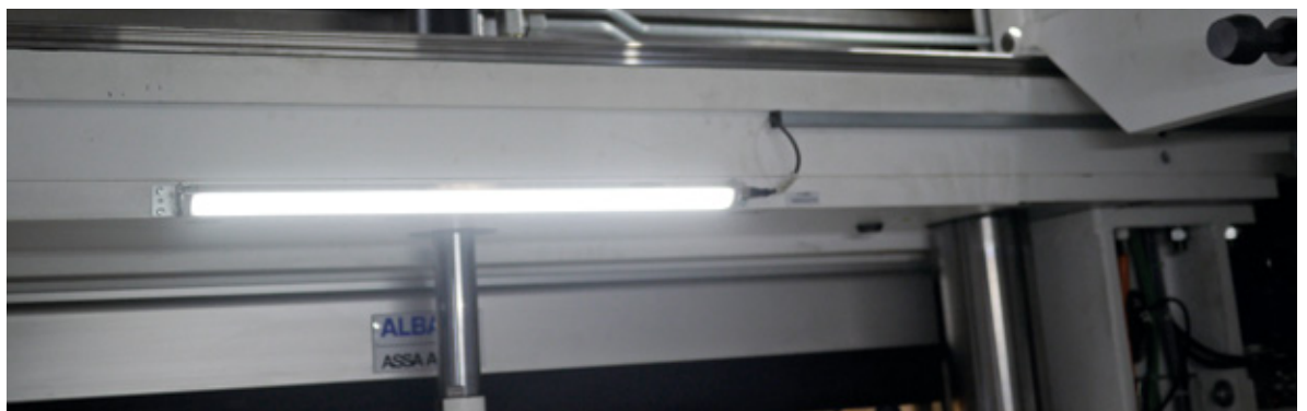
The WLS-28 dimmable LED machine light from the Turck portfolio is also connected with standard M12 connectors
