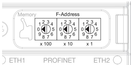
The module is delivered with the switch position 0. The address 0 and the addresses  $\geq 900$  are no valid F-addresses.
