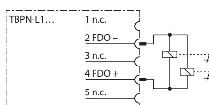
For PM-switching outputs, connect the negative pole of the load to the M-connector of the respective output (pin 2).
