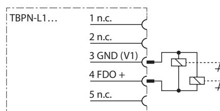
For PP-switching outputs, connect the negative pole of the load to the GND of the respective output (pin 3). Another connection to the GND of the power supply unit is not permitted!
