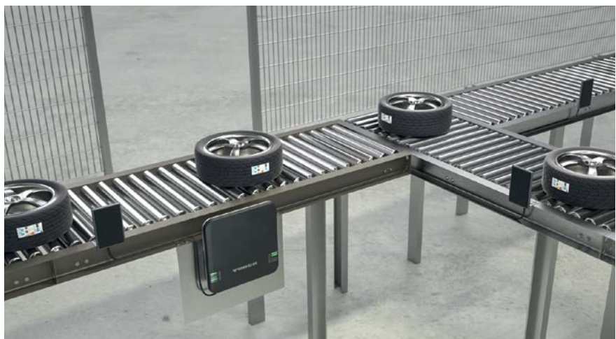
Detection of individual production goods on a conveyor belt
