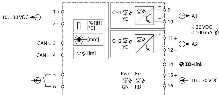
Fig.10: IM12-CCM03-MITS-3T-IOLC/24V...connection and wiring diagram
