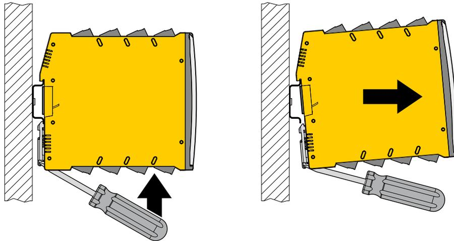
Fig.13: Dismantling the device — without power bridge connector
