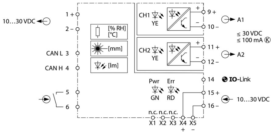
Fig.9: IM12-CCM03-MITS-3T-IOLC-PR/24V...connection and wiring diagram
