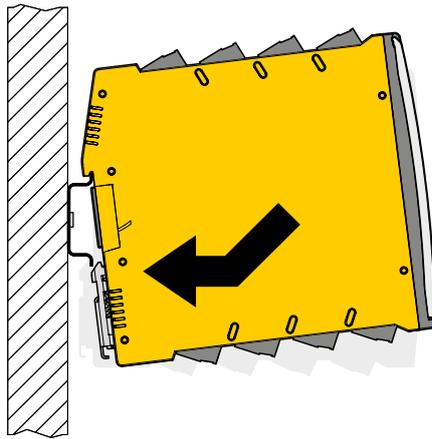
Fig.5: Mounting on a DIN rail
