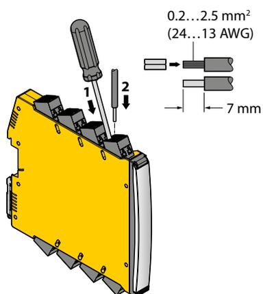
Fig.8: Connecting the device using spring-clamp terminals
