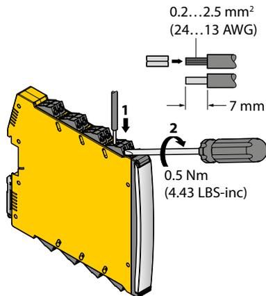
Fig.7: Connecting the device using screw terminals
