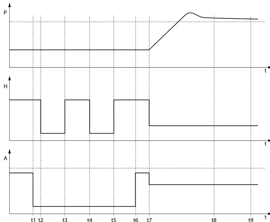
Fig.12: Teach function and tuning phase (P: fluctuating process variables such as temperature or humidity, H: brightness, A: distance value for door detection)
