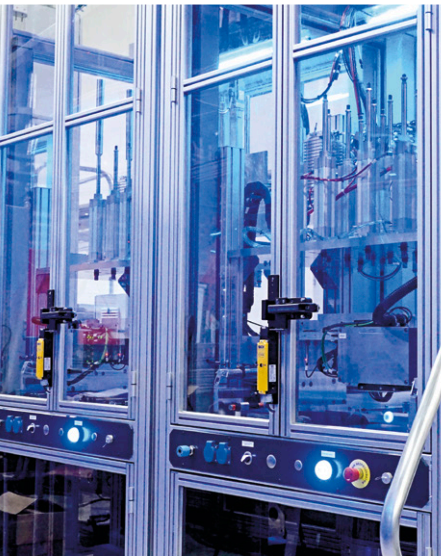
WLS27 LED line lights display the respective status of a module by color
